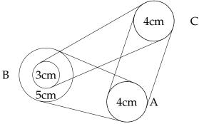
Connecting wheel C directly to wheel A means that wheel A should spin at the same speed as wheel C (because they have the same radius). However, we already saw that wheel C is spinning at 12rpm, and by royal decree wheel A spins at 20rpm. When a wheel has to spin at two different speeds, the system breaks down and all the wheels cannot move.
