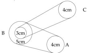
Wheel A is the input wheel, so it must move at 20 rpm. Then wheel B will move at  $20 \times \frac{4}{5} = 16$  rpm and wheel C will move at  $16 \times \frac{3}{4} = 12$  rpm.
